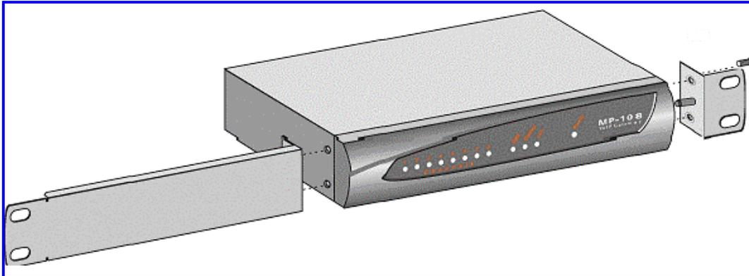
The **MP-10x** is installed into a standard 19-inch rack by the addition of the 2 brackets supplied, and shown above.
