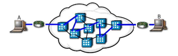
Phase 2 - Data-Transfer: Data is transmitted along the designated path of the network, arriving at the destination in the order it was sent.
