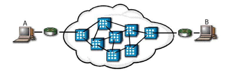
Phase 1 - Connection-Establishment: The source and destination negotiate a connection with a three-way handshake and a simple path between the two is determined.
