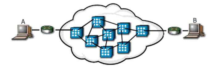
Phase 3 - Connection-Termination: The connection between the source and the destination is terminated when it is no longer needed. If they require additional communications after termination, another connection must be established.
