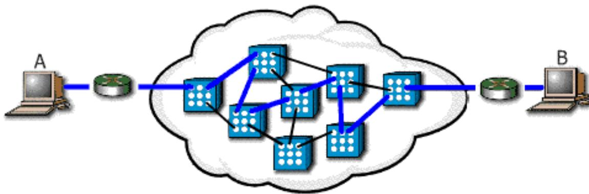
**Data Transfer: Next, data is transmitted between the DTE devices over the virtual circuit.**
