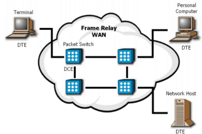
Frame relay network is not a single physical connection between endpoints. Logical paths are defined within the network. Based on the concept of using virtual circuits (VCs).
