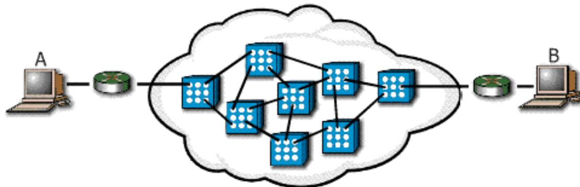
**Call Setup:** In this initial state, the virtual circuit between two Frame Relay DTE devices is established.
