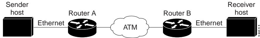
Figure 24 Example RSVP-ATM QoS Interworking Configuration
