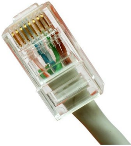
Figure 2-1. RJ45 connector with pinout (Photo copyright Georgios Alexandris | Dreamstime.com. )
